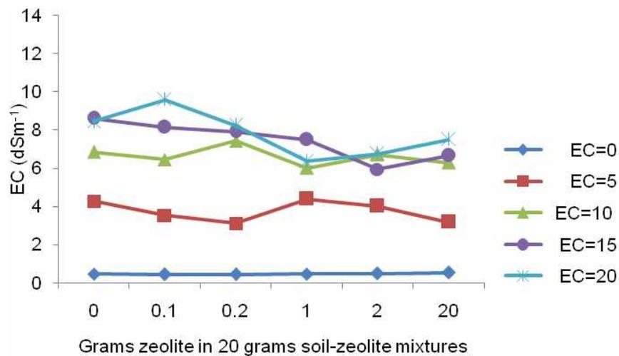
Figure 1. The effects of zeolite on electrical conductivity of soil using NaNO<sub>3</sub>
