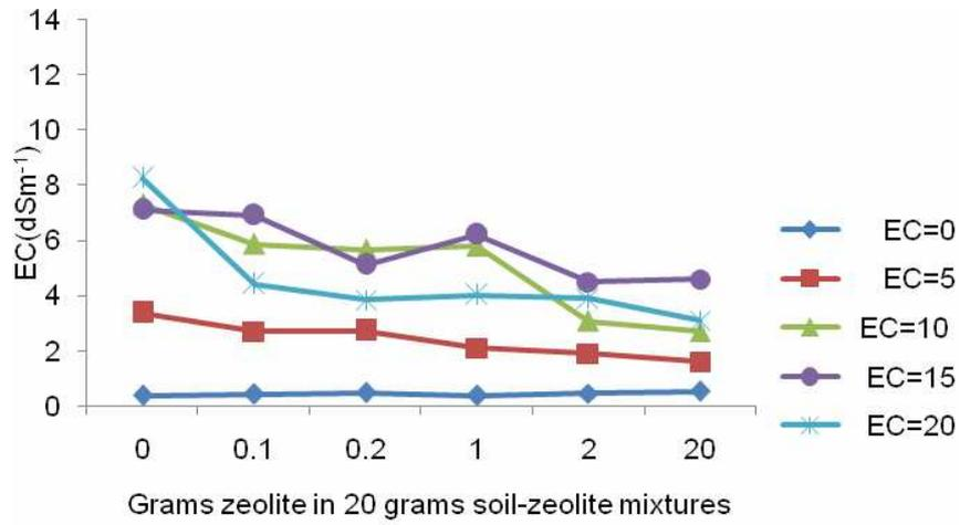
Figure 2. The effects of zeolite on electrical conductivity of soil using KNO<sub>3</sub>
