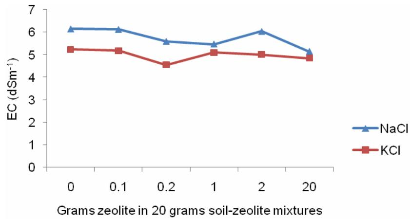
Figure 6. The effects of zeolite on electrical conductivity (pooled mean values for Na and K in chloride solutions)
