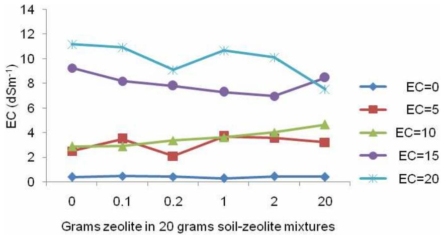
Figure 5. The effects of zeolite on electrical conductivity of soil using KCl
